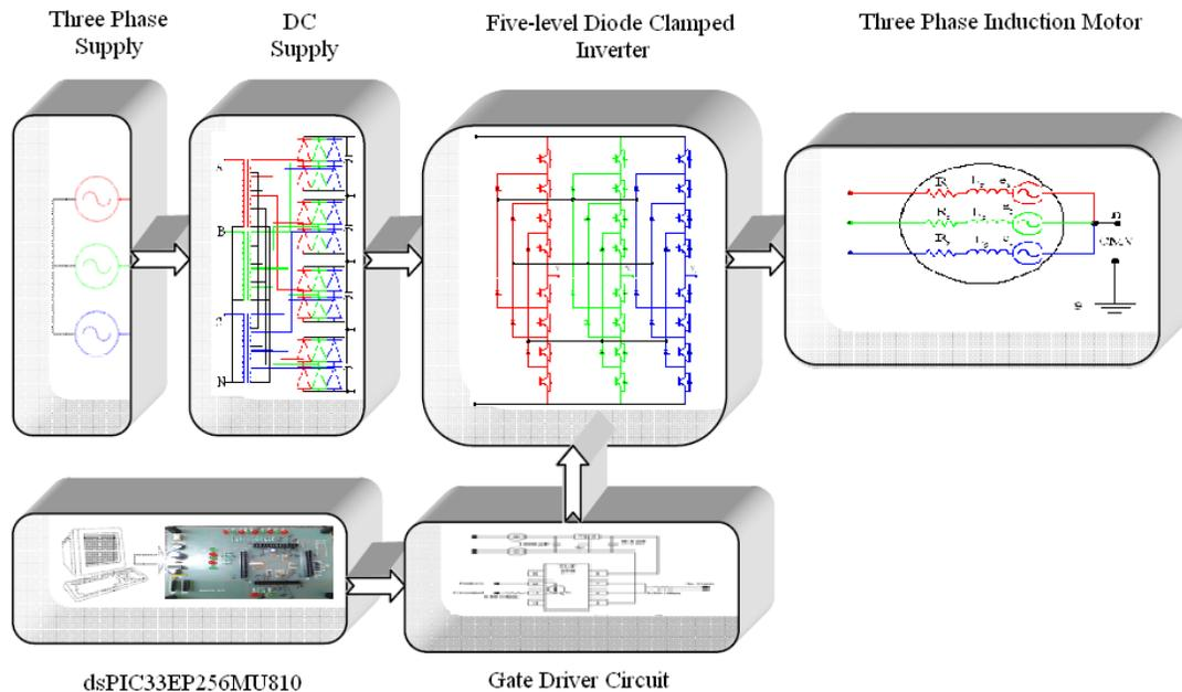
**INDUSTRY RELEVANCE :** The work is of great use to the industries where variable speed electrical drives are used. The life of the bearings can be increased with decrease in harmonics & rate of rise in voltage. It also reduces the ratings of the switching devices.
